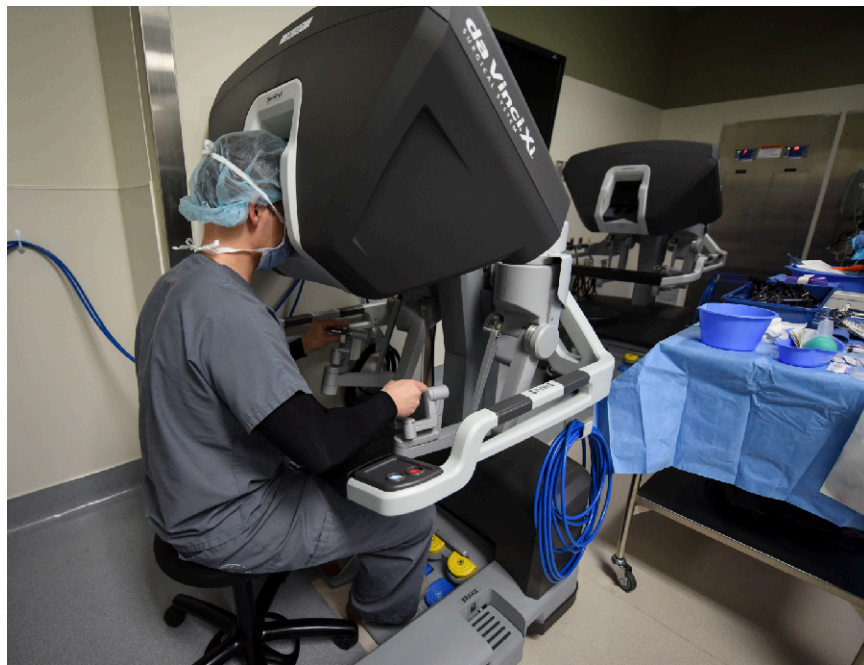
FIGURE 37.4 The Davinci Surgical System, a robotic surgical platform used for surgical procedures, is an example of how robots can enhance health-care delivery and patient outcomes. Artificial intelligence can help surgeons and equipment-makers analyze the performance on these machines and improve them over time. (credit: Air Force/Arnold Air Force Base, Public Domain)
