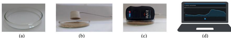
Figure 1 - Illustrative representation of the NIR spectra acquisition using a portable instrument. In portable instruments, (a) Petri dish, (b) Petri dish containing 20 cm 3 of sample, (c) MyNIR spectrometer, and (d) spectrum obtained by software.
