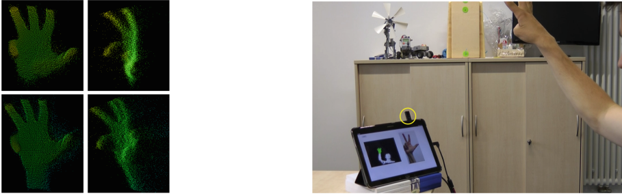
Fig. 1. Data and data generation. Left: Sample snapshot of a resulting point cloud after cropping from the front (left) and side view (right) during a grabbing motion. The lower snapshot describes the hand’s movement for each viewpoint (left and right respectively). Right: The Setup - tablet with a picoflexx (indicated with yellow circle). (Color figure online)
