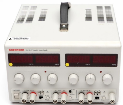
Figure 2.37 A multi-output adjustable DC voltage supply.
