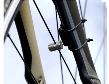
Figure 10.4 Bicycle computer sensor and magnet.
