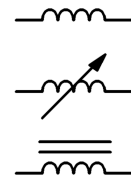
Figure 9.10 Inductor schematic symbols (top-bottom): standard, variable, iron/ferrite core.
