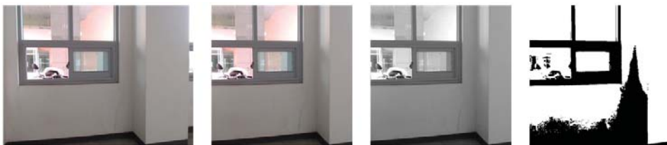
Figure 9. Convert process of original image. (a) Original image; (b) crop image; (c) gray-scale image; (d) binary image.
