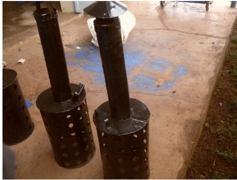
Figure 47: Open air carbonizers
