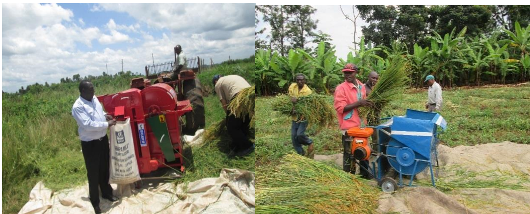
Figure 33: P.T.O. driven thresher (left) and motorized drum thresher fabricated at KALRO-Mwea
