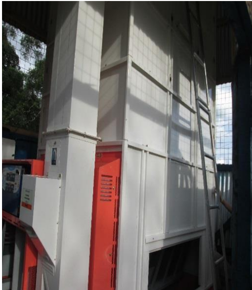
Figure 37: A recirculating air batch rice grain dryer at KALRO-Mwea
