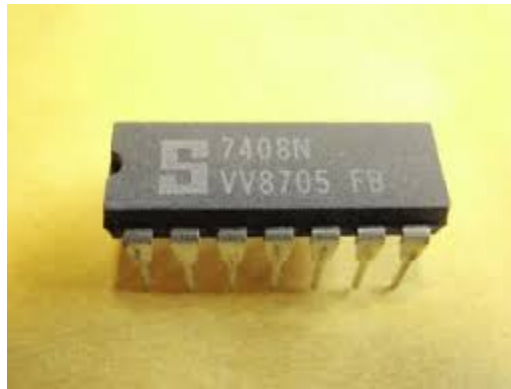
Figure 4-7: 7408 chip, notch indicates top of chip.
