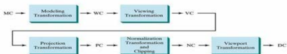
General three-dimensional transformation pipeline, from modeling coordinates to world coordinates to viewing coordinates to projection coordinates to normalized coordinates and, ultimately, to device coordinates.
