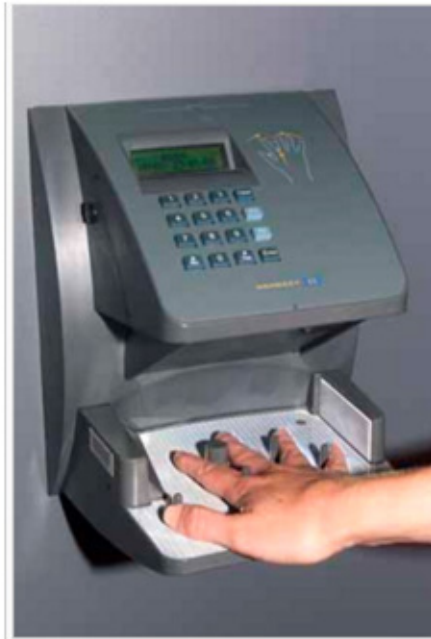
Physical security access control with a hand geometry scanner
