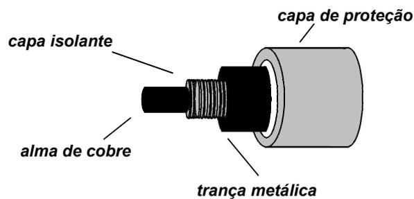
**Figura 2.3.1** - Cabo coaxial.
