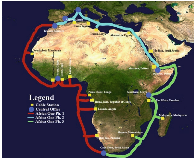
■ Fig. 12.5 Distribution model #2: The Bus or The Ring—Fiber network ring around Africa
